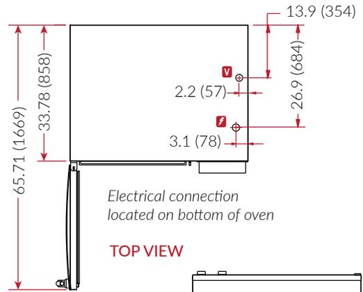
Electrical connection located on bottom of oven
